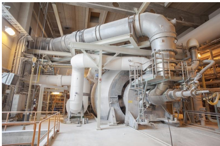
Biomass gasification with product gas feeding a multi-fuel lime kiln burner (typical plant)
